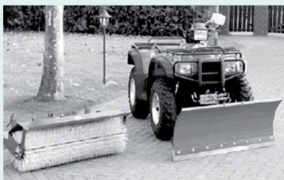
HONDA ATV with extra hydraulics
