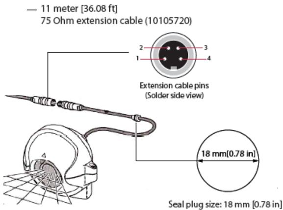
*Camera Connector Cable Pin Breakout*
